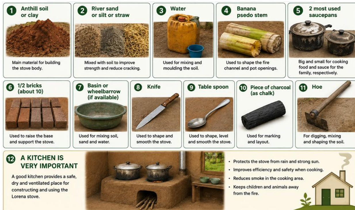
Figure 4.3: Materials for making a Lorena Stove
