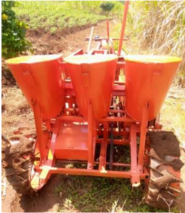
The adapted multi-row motorised planter-reduces drudgery and saves time
