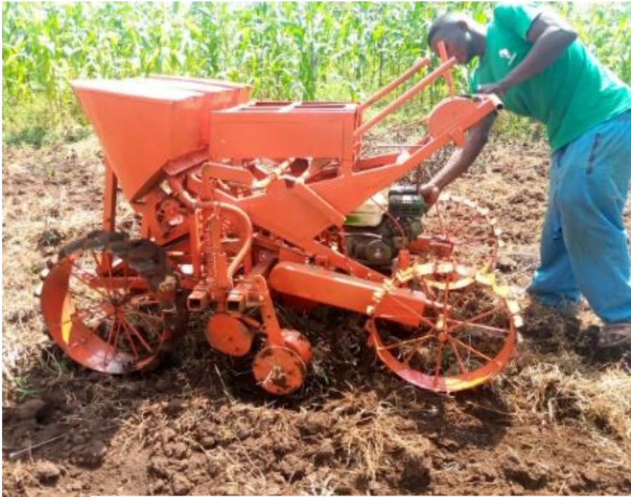
The adapted multi-row motorised planter-reduces drudgery and saves time
